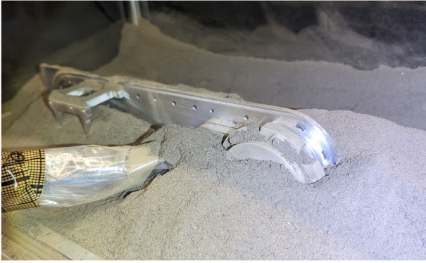
Figure 12: Drive Unit Regolith Sealing Testing (top), gear stages under Microscopic Imaging (Harmonic Drive / bottom left, spur gear stage / bottom right)
